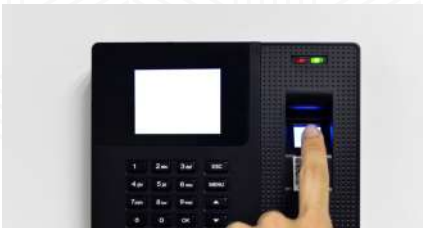
Biometric Access Control for lobby
